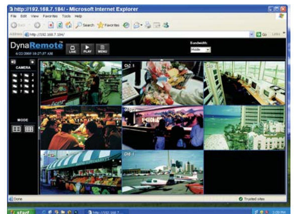
Users can remotely monitor, playback, change system settings, control connected dome cameras over a LAN or the Internet via the DynaRemote™ software
