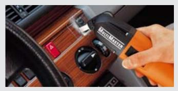
For sawing tasks in places that are not easily accessible or for small grooves. Cutouts from as little as 10 mm wide. Exceptionally suitable for all filing and sharpening tasks, in combination with the diamond file and the 15° clamping plate. This means it is ideal for all added fittings and installations.
