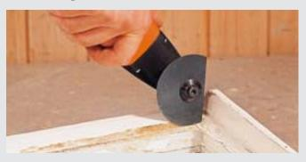
Use the saw blades to remove putty from single and multi-layered glazing without the risk of glass breakages and without laborious preparatory work.
