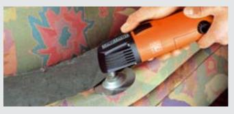
Ideal for upholsterers: sawing off and removing metal clamps with the cropped HSS saw blade.
