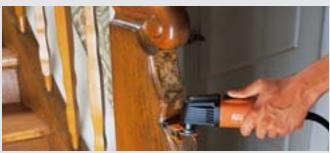
Six replaceable profiles of the profile sanding set enable you to sand cramped spaces, in grooves and on profiles – completely comfortable and with 300% improvement in sanding capacity. The flexible hollow sections perfectly adapt to various conditions.
