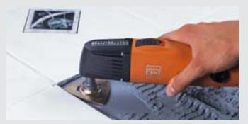
The carbide rasp produces optimum results when sanding down tile adhesive, sanding edges of tiles, coarse sanding wood, filler, paint and much more.
