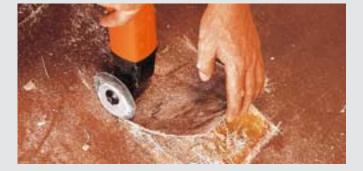
The HSS saw blades help you to saw fibreglass, carbon fibrereinforced plastic, wood and sheet metal up to 1 mm. Cropped saw blades enable you to work flush to the surface. The segment blades allow you to cut at right angles without overcutting.
