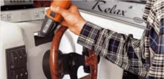
For sawing tasks in places that are not easily accessible, or for small grooves. Cutouts from as little as 10 mm wide. Exceptionally suitable for all sharpening tasks, in combination with the diamond file and the 15° clamping plate.
