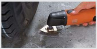
Remove oil patches from garage floors, graffiti from concrete and stone facades or other unwanted remains using the tungstencoated rasp.
