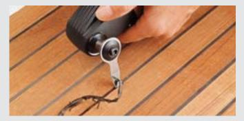
The cutter blade ideal for rapid and secure cutting out of panelled deck sealing materials is also suitable for problem areas such as cabins, rails, gunwales, cleats and curves.
