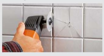
Use the diamond saw blade to cut out marble and concrete trass joints as well as to make grooves in plastered walls, dry wall, sheet rock, porous concrete.
