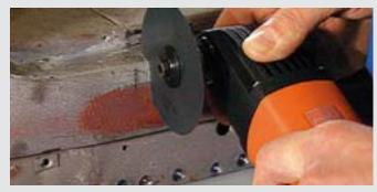
Use the HSS saw blade for sawing sheet metal up to 1.0 mm, wood, putty, carbon fibre and fibre-reinforced plastic. Cropped saw blades enable you to work flush to the surface.
