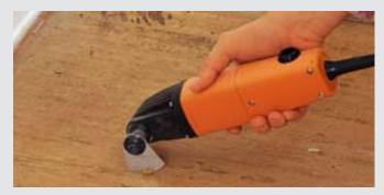
Use the segment blade for cutting rigid materials, e.g. floor coverings of plastic, rubber, cardboard, leather, woven wire cloth, loop pile carpet and other carpet, and much more.
