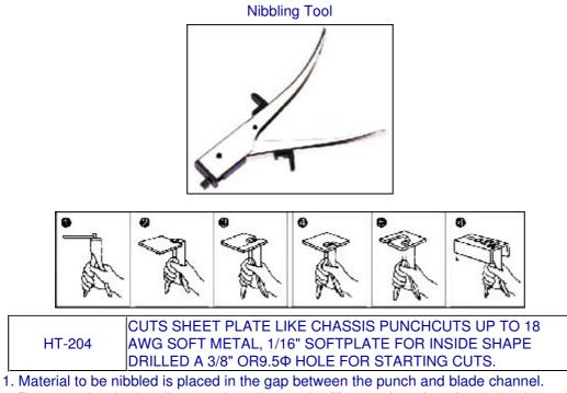
2. By squeezing the handles together, the punch will move down into the channel, cutting out a slug of metal.
