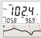
Using the record function, it is possible to check the amplitude of fluctuations.
