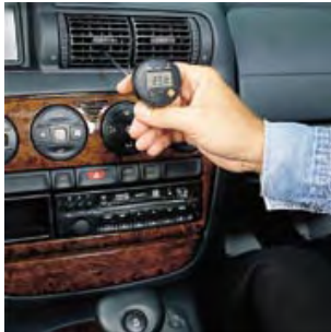
Measurements on air conditioning systems
