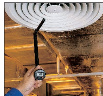
Measures air velocity in a ventilation duct
