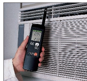
Measuring the air velocity at the outlet of a ventilation unit
