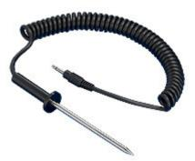
The 80PR 60 probe expands the utility of your RTD non-contact infrared thermometer by allowing you to take contact temperature readings. You can make contact and non-contact readings at the same time because your RTD infrared thermometer displays the results of both. Just plug the temperature probe into the RTD jack, position the probe tip at or below the surface of your target, and start reading temperatures. (Refer to thermometer user manual for details.)
