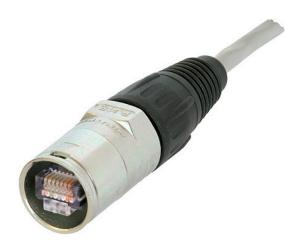
Cable connector carrier consists of a shell, fixing disk, chuck and bush. The boot (same as X-Series) is suitable for cable diameters from 3.5 - 8 mm. For non preassembled cables only. Cable connector carrier does not include a RJ45 plug.
