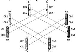
Upper and lower beams should be the same model type in stacked configurations.
