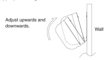
4. Hold the receiver and perform fine tune on right or left.(Horizontal adjustable angle is  $\pm 10^{\circ}$ )
