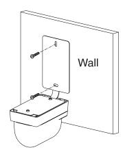
3. Hold the receiver and bend the bracket upwards. Adjust the receiver to appropriate angle to make the receiver's front position face the venue.
