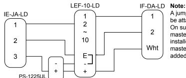
A jumper between E & - must be attached on the master. On surface/desk mount LEF masters, the jumper is factory installed. On LEF-C series masters, the jumper must be added.
