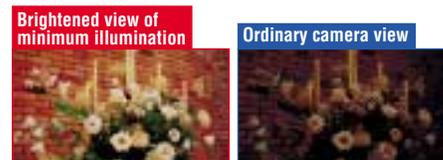
\*The image tends to blur more than that in standard mode when viewing a moving subject in low light or when using the pan, tilt, or zoom function. (Minimum illumination: BB-HCM381A, KX-HCM280A: 0.09 lux, BB-HCM311A, HCM331A, HCM371A: 0.2 lux)
