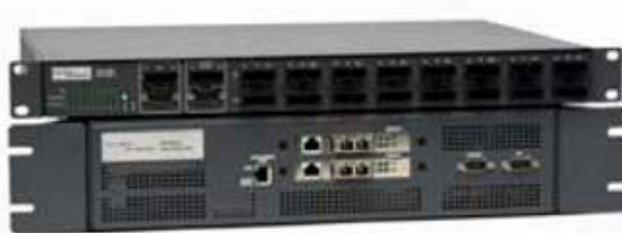
*OptiView Link Analyzer (OPV-LA) with a 8-port Fiber Top (FTAP-8M)*
