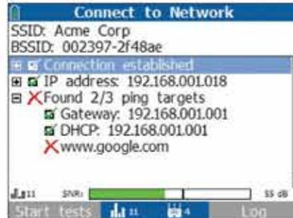
View the process steps on the display and store them in a log for troubleshooting. Quickly test performance and quality of the connection by using the continuous ping response, loss-rate, and connection-range features.
