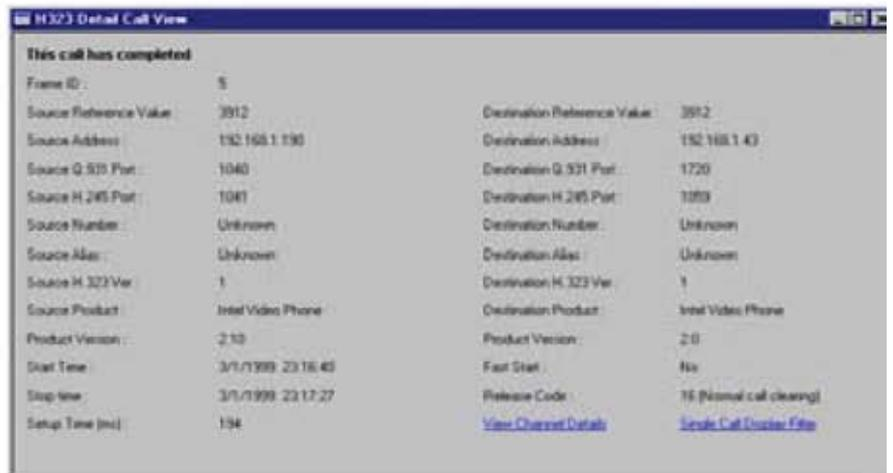
*H.323 Detail Call View shows real-time key call setup parameters using H.323 protocols. Similar tables are available for calls initiated using SIP and SCCP.*
