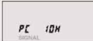
Figure 4. 10 Base-T signal detected, wired to PC.
