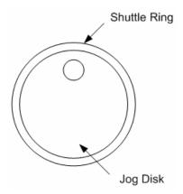
While playing back recorded video, users can rotate the shuttle ring to select different speed of forward and backward playback. Rotating the shuttle ring clockwise/counterclockwise causes the unit to playback faster forward/ backward. According to the rotating angle the shuttle ring, users can choose the playing speed from 1×, 2×, 4×, 8×, 16×, and 32×, in both forward and reverse directions, shown as below figure:
