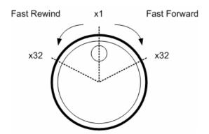
Inside the shuttle ring is the jog disk, shown as below figure. It can turn in either direction. Once the video is paused, users can use the jog disk to playback by single-step. Clockwise rotation causes a forward one-step playback; and counterclockwise rotation causes a backward one-step playback.
