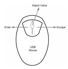
For example, if users want to change dome camera ID, enter the OSD setup menu with an authorized account and go to the following path: <Camera> → <Dome ID>.
