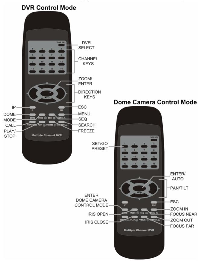
The keys of the remote control function as the keys of the front panel of the DVR. The only difference between the remote control and the front panel is the "DVR SEL" key. The DVR Selection key is used to switch control between different DVRs.
