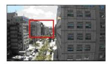
Up 10 Motion Detection Windows can be set. Click on the <add> button under the Live Video Pane to add a Motion Detection Window. To cancel a Motion Detection Window, move the mouse cursor to the selected Window, and click on the <delete> button.
